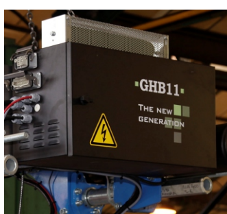
17 / Hoist electric cabinet
