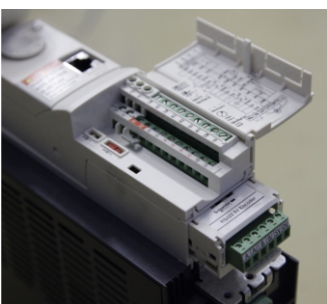
11 / Hoist Frequency inverter
